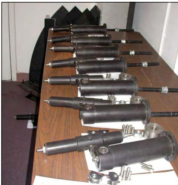
*The primary mirror side supports were removed from the VATT in 2006 for cleaning and evaluation.. (Photo by C.Corbally, S.J.)*
