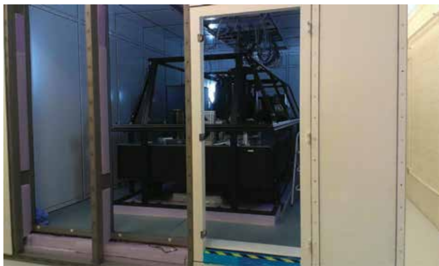
The PEPSI spectrograph being reassembled in its enclosure where it will be kept in a stable atmosphere at a constant temperature with variations less than one thousandth of a degree (Credit: M. Steinmetz).
