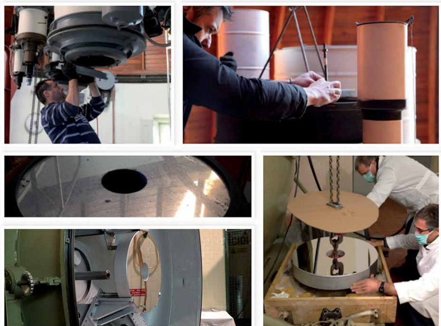
Images of VO staff dismantling the Zeiss mirror. The mirror was later re-aluminized by Asiago observatory staff.
