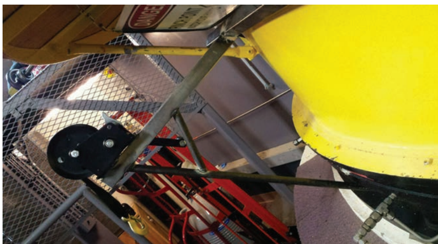
Winching system for safe instrument changes of VATT's spectrograph
