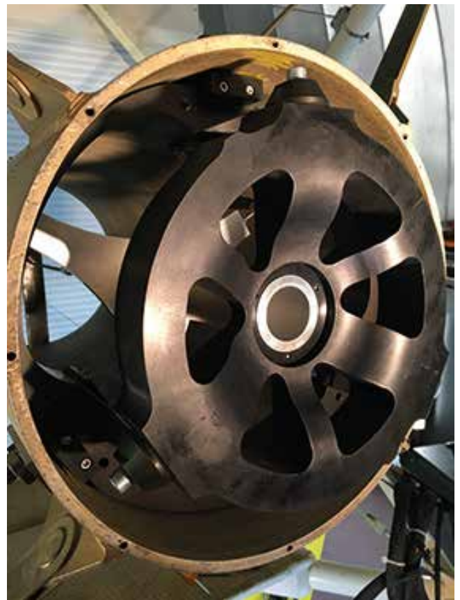
Isogonic mechanical interface with handling implement in M2's baffle barrel. View in the direction towards M1
