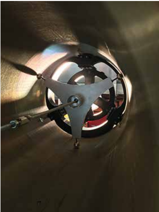
Isogonic mechanical interface with handling implement in M2's baffle barrel. View in the direction away from M1
