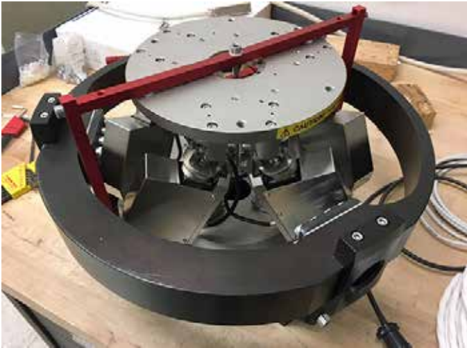
PI H-824 mounted inside the isogonic mechanical interface
