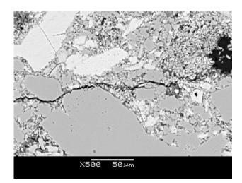
An electron microscope image of a rock obtained near a terrestrial impact site shows that the force of the impact creates cracks and voids in the rock. These cracks may be large enough to shelter microbes, suggesting such life forms could travel through space inside meteorites. (Image by Sara Russell, Natural History Museum of London, and Guy Consolmagno, S.J.)
