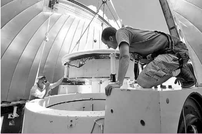
Ned Franz and Chris Johnson guide the VATT's primary mirror back into its cell after it was successfully re-aluminized during the summer maintenance shutdown.
