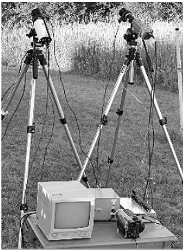
Camera set-up to record micrometeoroids.
