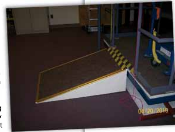
• Ramp to load the vacuum pump and instrumentation safely onto the scissors lift and up to VATT telescope. Photo: Gary Gray • The Vatican Observatory Jeep buried after a week of severe snow storms, January 2010. Picture taken from the safety of the Bannan Astrophysics Facility and before the MGIO crew rescued it so the photographer could leave the mountain. Photos: Richard Boyle
