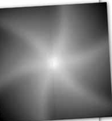
• In order to measure the brightness of stars accurately to one part in a thousand, it is necessary to know exactly how long each part of the image has been exposed. Stott's work, illustrated here, shows that the motion of the camera shutter slightly overexposes some parts of the image compared to other parts, and allows him to account for this variation from place to place on the image itself. Photo: Jonathan Stott
