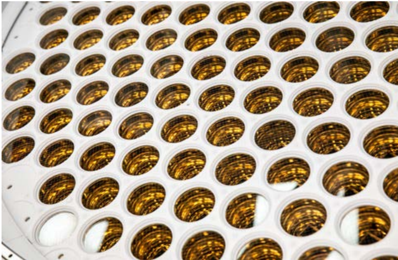
Top: LUX-ZEPLIN scientists inspect the Xenon Detector for dust. Bottom: The photosensor array for the LZ detector (photo credit: M. Kapust, SURF)
