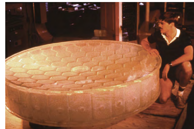
The mirror of the VATT as it was formed with a parabolic surface in the rotating furnace
